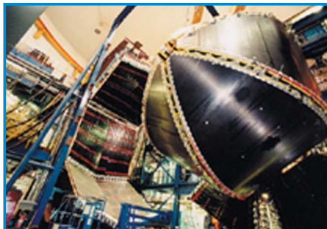
The Hall B CEBAF Large Acceptance Spectrometer (CLAS) at Jefferson Lab. It completely surrounds its target and collects up to a terabyte of data per day.
