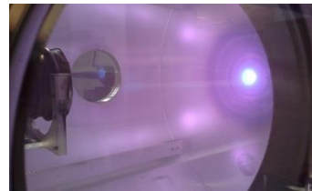
Fig 9 Plasmoids in Argon plasma with severity that corresponded to that of the arc. In previous Helium arcs the IPG heat loss spiked while the calorimeter heat loss dipped. With Argon, both spiked. Thus during this arc, RF power that is usually not transmitted to either the calorimeter or to the IPG was diverted.
