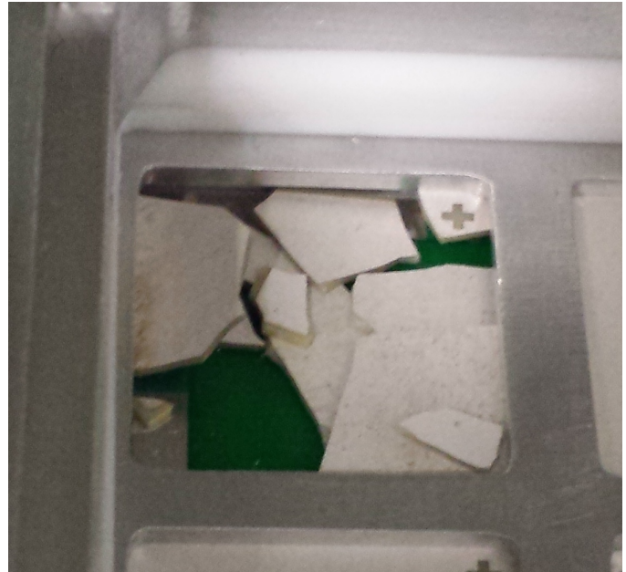
Fig. 14. Repeatedly Broken PZT
