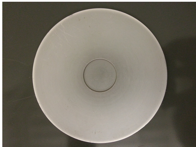
Fig 1. This is a view of a dish with a 1 mm deep and 25.4 mm diameter cutout.
