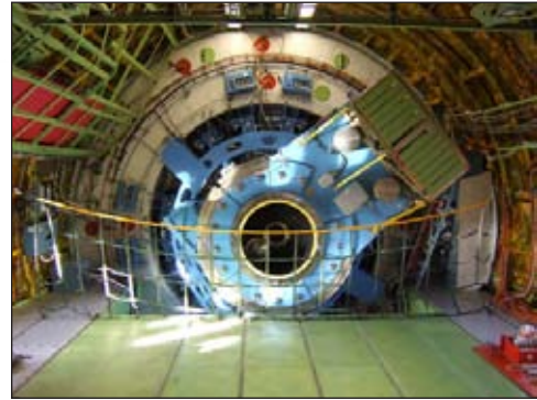
The 45,000-pound infrared German Aerospace Center telescope assembly inside the SOFIA aircraft.
